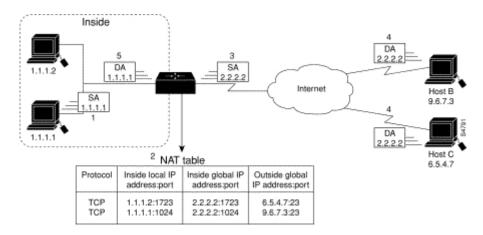
Figure 2- 2 NAT Operation During the Reloading of Inside Global Address
