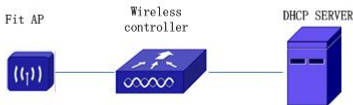
Fig 6- 1 Typical DHCP option 60 and option 43 topology
