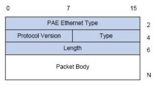
Fig 2- 3 the Format of EAPOL Data Packet
