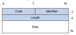
Fig 2- 4 the Format of EAP Data Packets
