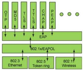
Fig 2- 8 the Protocol Stack of EAP Authentication Method
