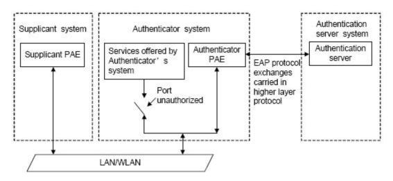
Fig 2- 1 The Authentication Structure of 802.1x
