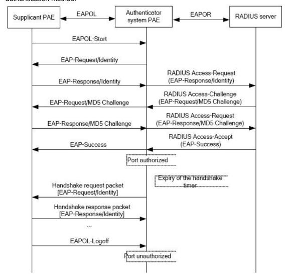
Fig 2- 9 the Authentication Flow of 802.1x EAP-MD5
