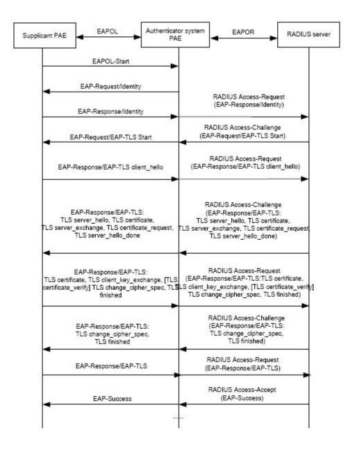
Fig 2- 10 the Authentication Flow of 802.1x EAP-TLS
