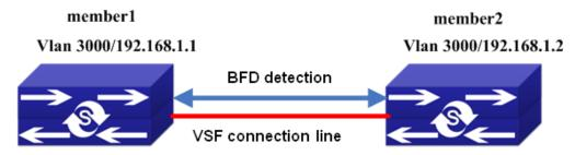
As show in the above picture, assume the ports used for bfd mad detection are ethernet1/1/1 and ethernet2/1/1, and the vlan is 3000. The configuration of mad ip address is the network segment of 192.168.1.1 for example.
