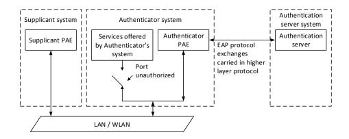
Figure 46.1: The Authentication Structure of 802.1x
