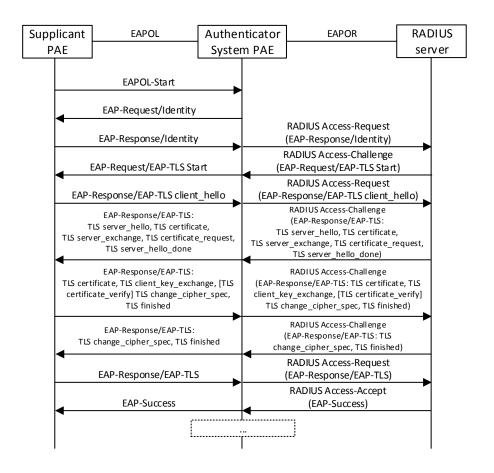
Figure 46.10: the Authentication Flow of 802.1x EAP-TLS
