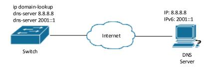
Figure 68.1: DNS CLIENT typical environment
