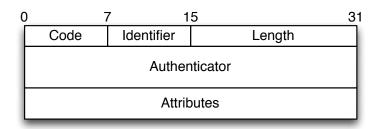
Figure 51.1: Message structure for RADIUS
