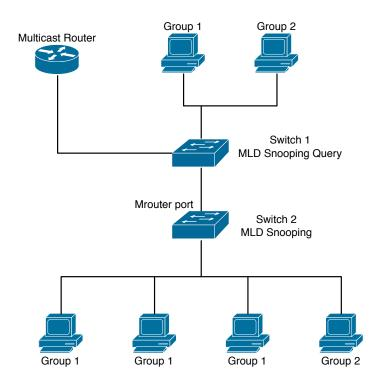
Figure 43.2: Switch as MLD Querier Function figure
