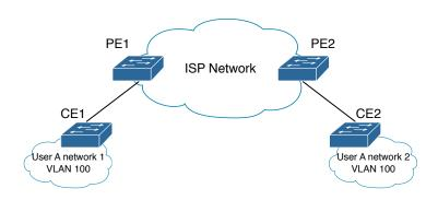
Figure 16.1: BPDU Tunnel application
