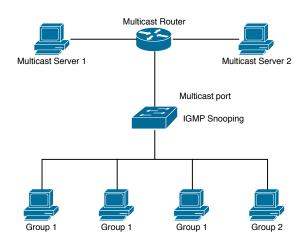
Figure 42.1: Enabling IGMP Snooping function
