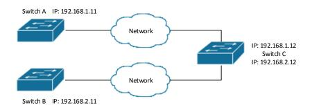
Figure 67.1: Typical NTP Example
