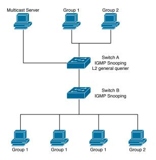
Figure 42.2: The switches as IGMP Queries
