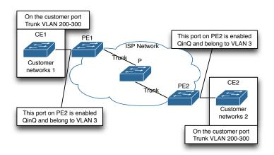
Figure 19.1: Dot1q-tunnel based Internetworking mode
