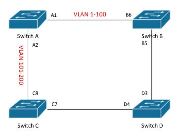
Figure 60.2: VLAN load balance
