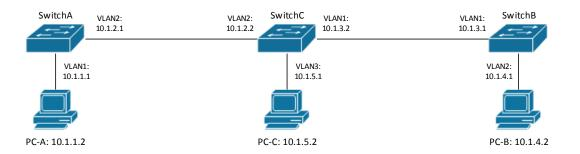
Figure 31.1: Static Route Configurations
