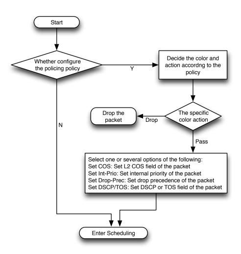
Figure 28.6: Policing and Remarking process
