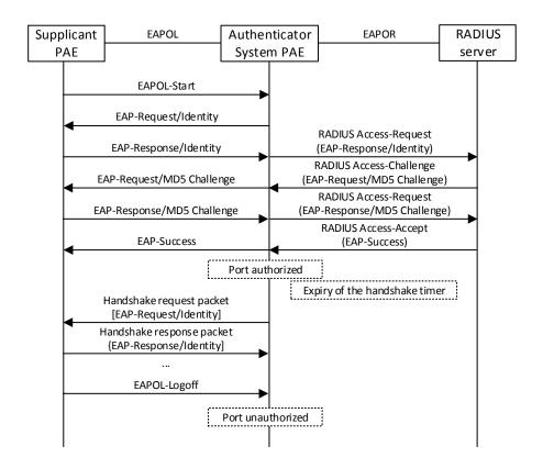
Figure 46.9: the Authentication Flow of 802.1x EAP-MD5
