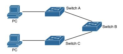
Figure 24.2: Typical GVRP Application Topology
