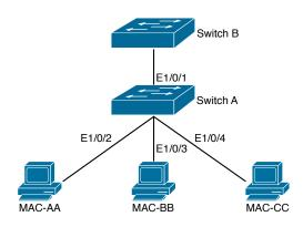
Figure 40.1: DHCPv6 Snooping option schematic
