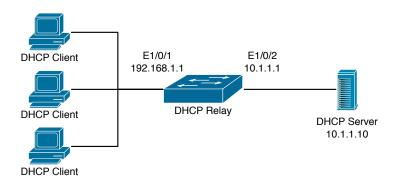
Figure 36.3: DHCP Relay Configuration
