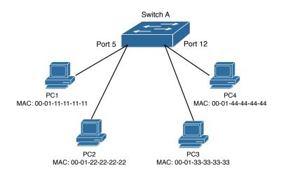
Figure 26.2: MAC Table typical configuration example
