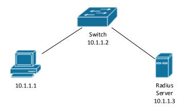
Figure 46.16: IEEE 802.1x Configuration Example Topology
