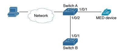
Figure 15.1: Basic LLDP-MED configuration topology
