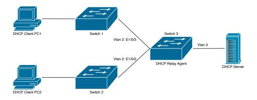
Figure 38.2: A DHCP option 82 typical application example
