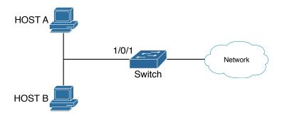
Figure 13.1: Typical topology chart for port security
