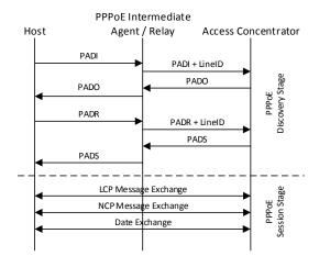
Figure 55.1: PPPoE IA protocol exchange process
