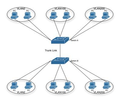
Figure 18.2: Typical VLAN Application Topology
