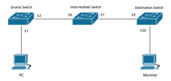
Figure 64.1: RSPAN Application Sample
