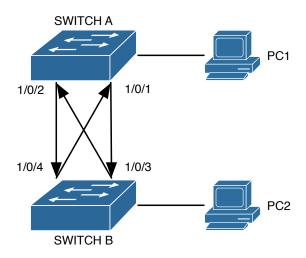
Figure 8.3: Fiber Cross Connection
