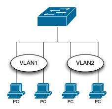
Figure 57.1: VLAN-ACL configuration example
