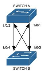
Figure 8.1: Fiber Cross Connection
