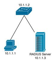
Figure 51.2: The Topology of IEEE802.1x configuration
