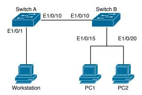
Figure 44.1: Function configuration of the Multicast VLAN
