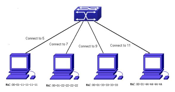
Fig 2-2 MAC Table typical configuration example
