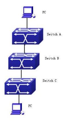
Fig 1-5 Typical GVRP Application Topology
