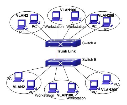
Fig 1-2 Typical VLAN Application Topology
