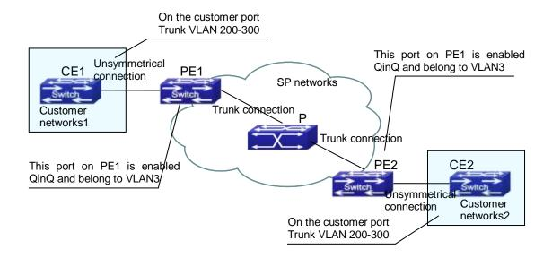
Fig 1-6 Dot1q-tunnel based Internetworking mode
