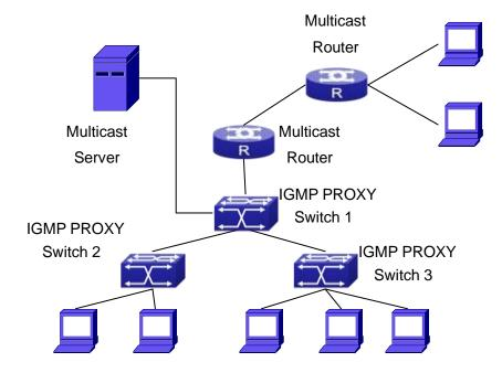
Example2: IGMP Proxy for multicast sources from downstream ports.
