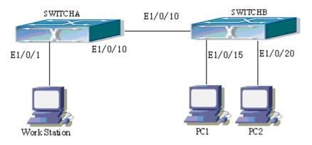
Fig 3-1 Function configuration of the Multicast VLAN
