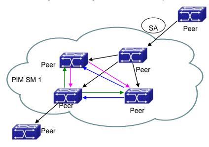
Fig 1-4 Flooding of SA messages
