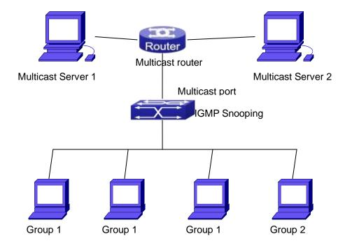
Fig 1-10 Enabling IGMP Snooping function
