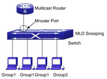
Fig 2-6 Open the switch MLD Snooping Function figure
