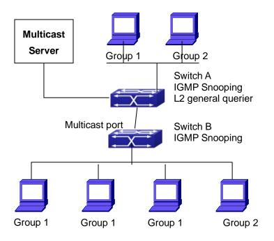
Fig 1-11 The switches as IGMP Queries
