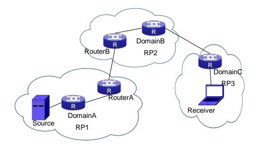
Fig 1-3 Network Topology for MSDP Entry
