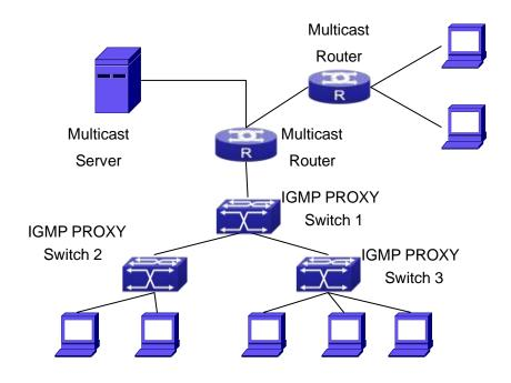
Fig 1-12 IGMP Proxy Topology Diagram
