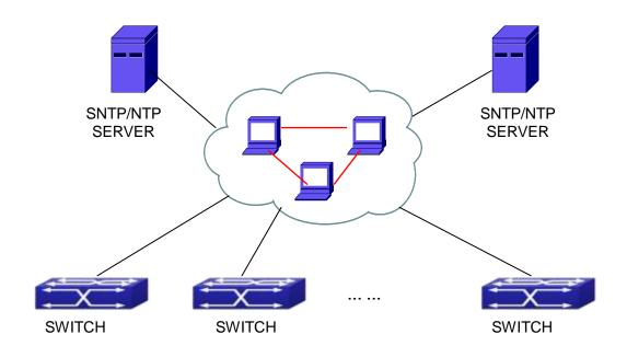
Fig 1-2 Typical SNTP Configuration
